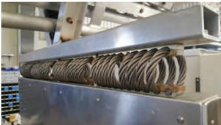
**Vibration Isolation** - Aluma's engineering team worked with a Harmonics Engineer to specify coil and cup isolators for each major component of the system, this was done to prevent damage to components during transport on un-improved roads. Special attention was given to the radio cabinet, generator, tower, fuel tank, storage box, etc.
