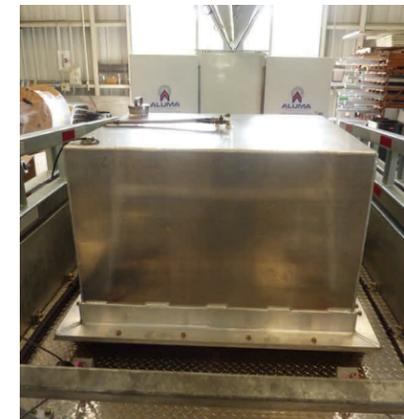
**Fuel Tank** - Double-walled all aluminum fuel tank with baffles strategically placed to support over 200 Gal's of Fuel. Mounted on vibration isolators and located over the trailer axles to improve balance of the overall system. Designed to meet all FMCSA requirements, the pressure tested fuel tank is a unique feature that can be adjusted to meet customer specifications. A 200 gal. tank can provide fuel to small generator for a 2 week uninterrupted period.
