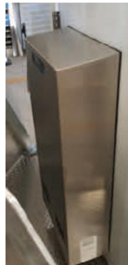
**ECU Isolation Package** - Aluma's engineering team worked directly with the manufacturer of the radio cabinet ECU to design a vibration isolation package for the internal components of the unit. The ECU on the "Super Scorpion" has built in isolators that isolate the internal components from the ECU housing.
