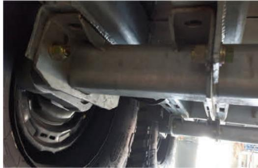
**Double Bracketed Torsion Axles** - While the baseline system included torsion axles, they are traditionally only supported by a single bracket on the road and curb side of the system. The updated design provides twice the bracket locations increasing the reliability, safety and structural integrity of the axle system. This new Axle bracket is design specifically to survive through the most harshest of road conditions.
