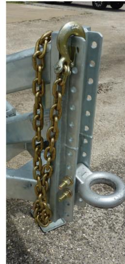
**Adjustable Tongue Height & Multiple Voltage Electrical Brakes** - The tongue incorporates a larger channel and additional bracing that allows for coupling from multiple vehicles, taking into consideration hitch heights of various commercial and military trucks. The total adjustable range of the coupler is 18 1/2 to 38 1/2 inches. The "Super Scorpion" is also armed with a 4 wheel electrical brakes capable to be used by 12V or 24V military and any commercial prime mover
